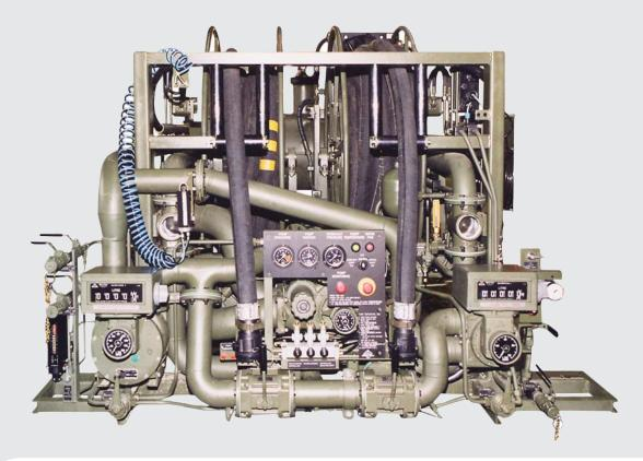
The Tactical Aircraft Refueller ART with the Aircraft refuelling unit ARU 1350 is used for refuelling of helicopters and vehicles with aviation fuel from own tank.
