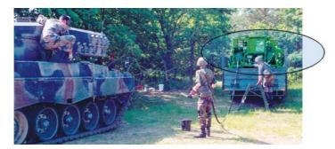
**Truck- or Tank-Refueling** 2 x 200 l/min with nozzle KPA 400 B stand alone mounted on a light truck
